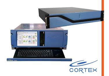
Safran Data Systems Best Source Selector (BSS) is the perfect tool to select the best Telemetry source received from multiple antennas tracking the same airframe, carried through different medias, in real time.
